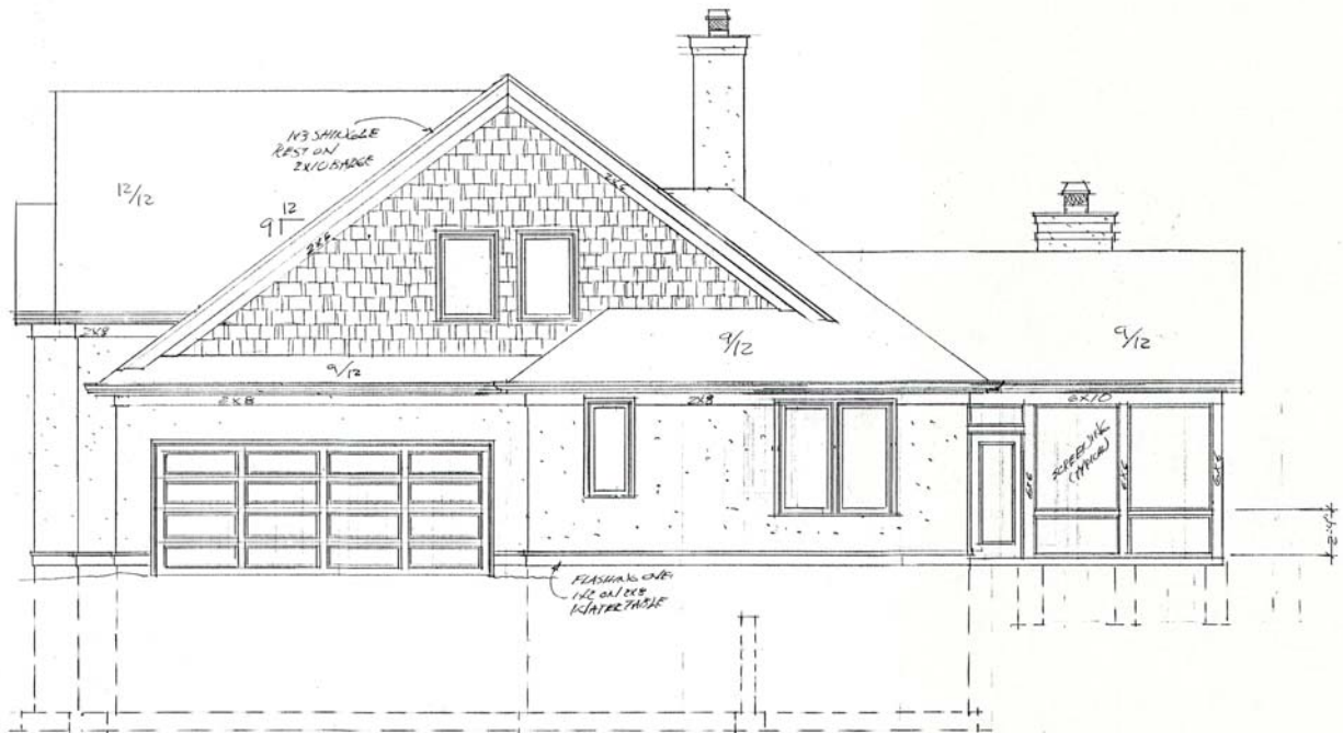
LEFT SIDE (WEST) ELEVATION SCALE 1/4" = 1'-0"
