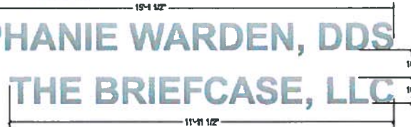
B Letter Detail SCALE: 1/2" = 1'-0" 1/4" thick flat-cut aluminum letters, brushed aluminum paint finish. Pin-mount 1" from surface with spacers. Arial Bold font.
