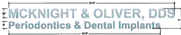
B Letter Detail SCALE: 1/2" = 1'-0" 1/4" thick flat-cut aluminum letters, brushed aluminum paint finish. Pin-mount 1" from surface with spacers. Arial Bold font.
