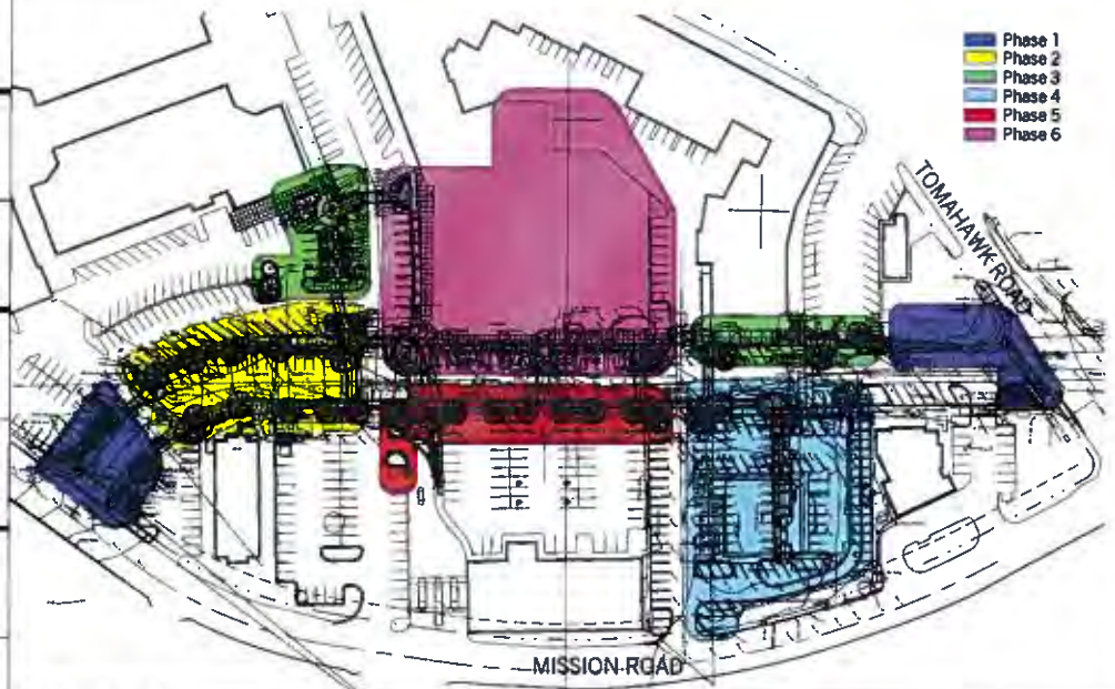
A1 Scale 1" = 60'-0" Construction Phasing Plan
