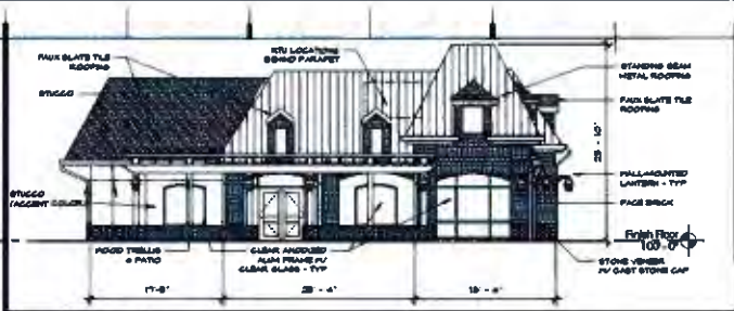
L9 Scale 1/8" = 1'-0" Exterior Elevation - West
