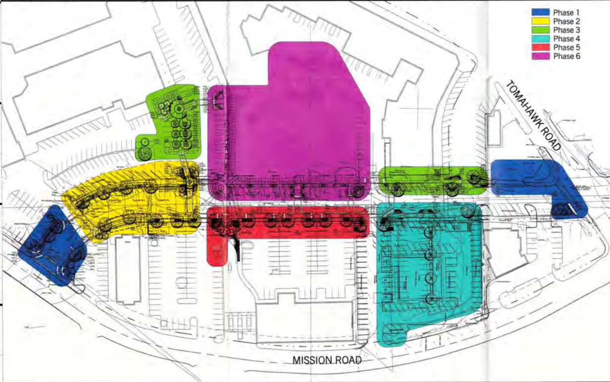
1 Scale 1" = 50'-0" Construction Phasing Plan
