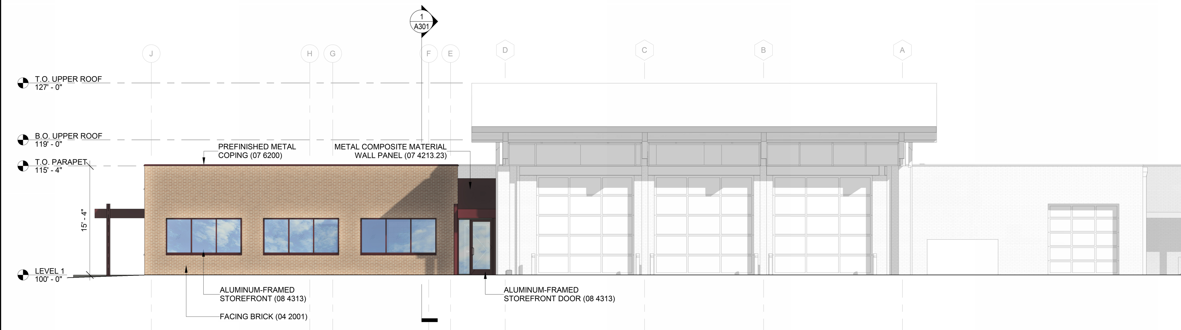
B1 EXTERIOR ELEVATION - NORTH A201/ 1/8" = 1'-0"
