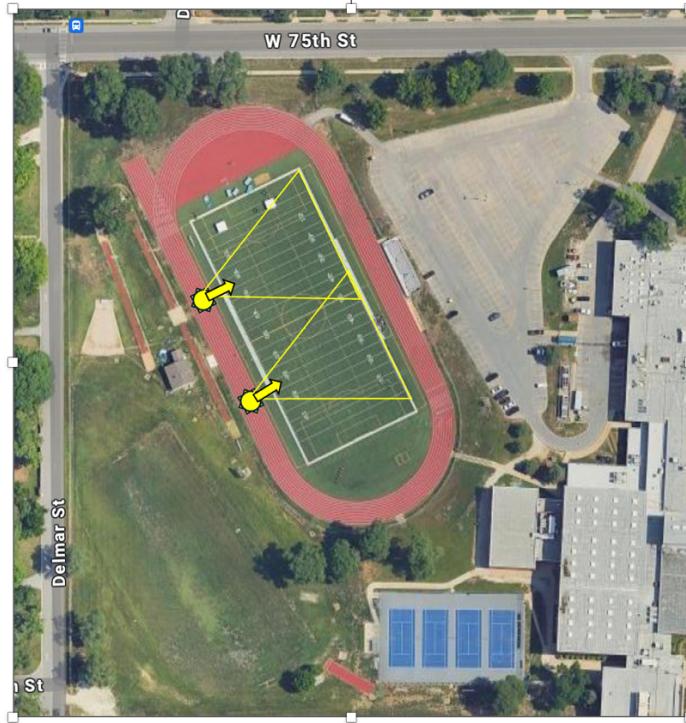
Sample Temporary Lighting Orientation with 2 lights
