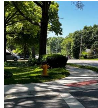
Figure 3: Intersection Sight Distance Blockage
