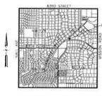
Unadjusted Error of Liosure of Error Distance: 0.003 North: 0.0009\* Eost 0.0028 Perimeter 614.50
