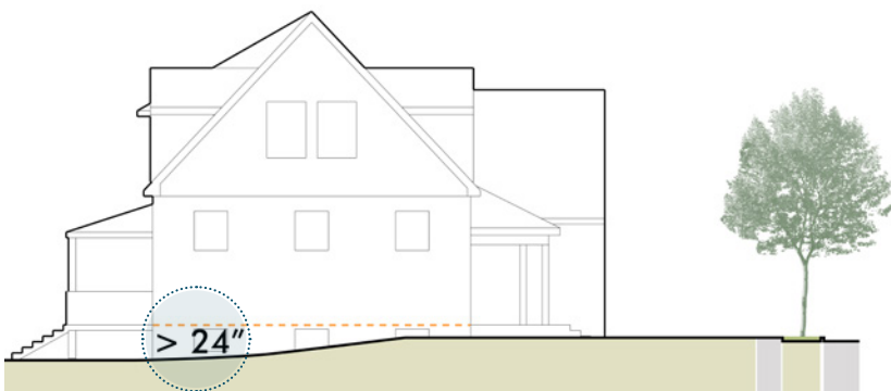
Building Foundation: more than 24" of foundation exposed due to grade changes
