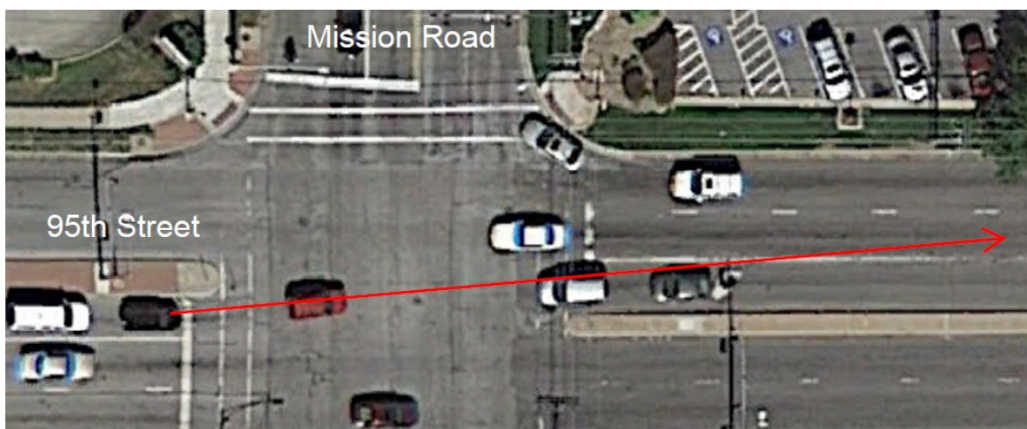
Queued vehicles in the westbound left-turn lane block an eastbound left-turn driver's view of opposing through traffic at 95th Street and Mission Road
